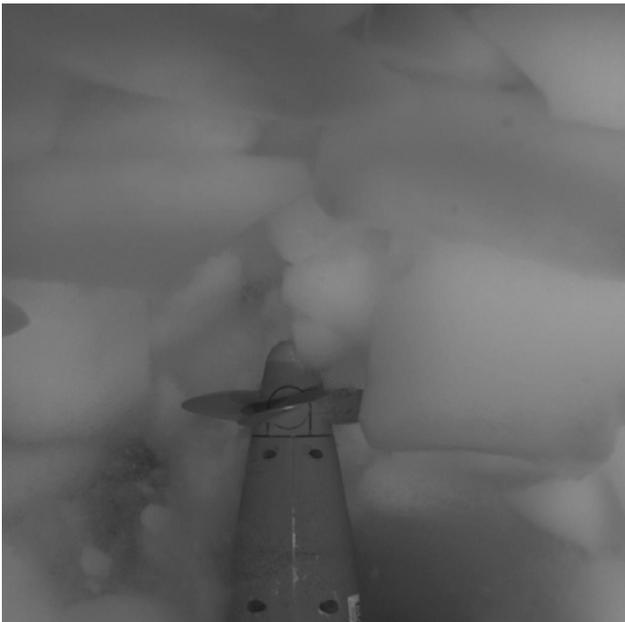
Figure 13: still from high speed camera with propeller entering an ice ridge
