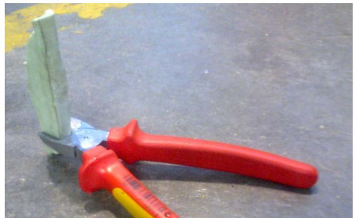
Figure 7: foam for the ‘foam-hammer’ test
