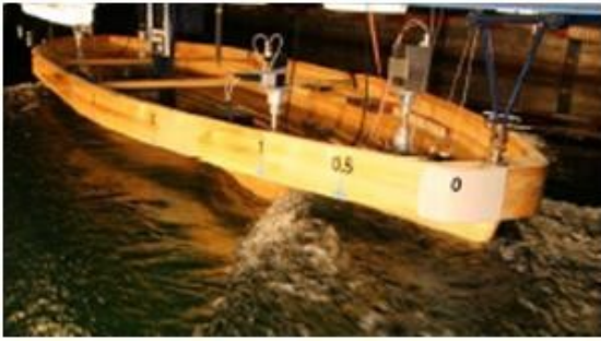
Figure 11: Wave system from AFT thruster head box
