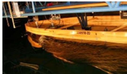
Figure 10: Wave system from FWD thruster head box
