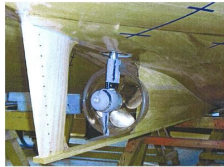
Figure 4: Single ducted thruster unit arrangement
