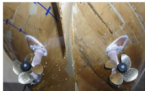
Figure 6: Twin (wing) thruster units arrangement
