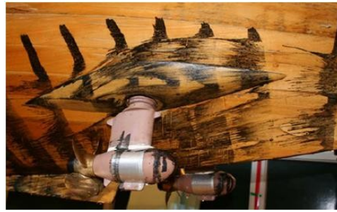
Figure 8: Illustration of a thruster head box under paint streamline test
