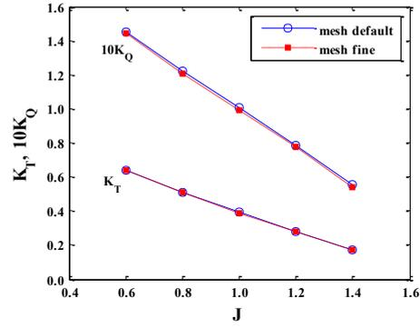
Figure 4: Propeller performances (non-cavitating)
