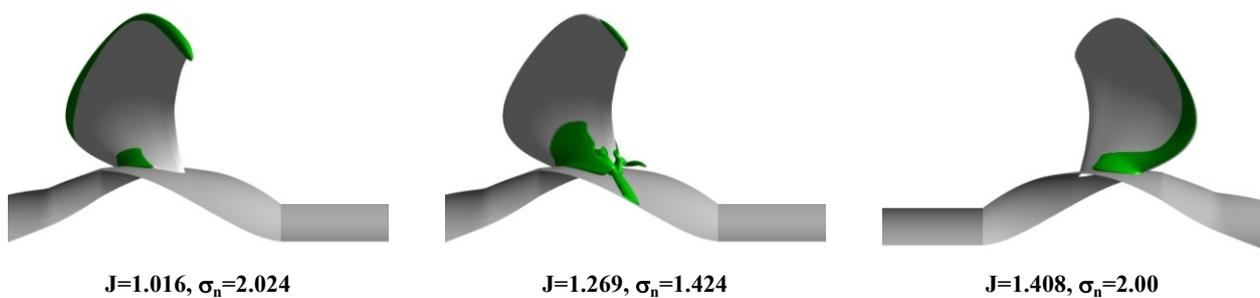
Figure 10: Cavitation patterns depicted as isosurfaces of vapour volume fraction  $\alpha=0.20$  obtained using the Zwart model.
