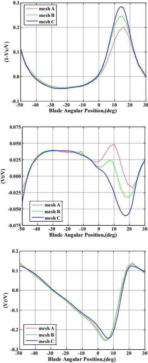
**Figure 8: Velocity profiles computed in a plane  $x/D=0.2$  downstream of the propeller mid plane at  $r/R=1$ .**
