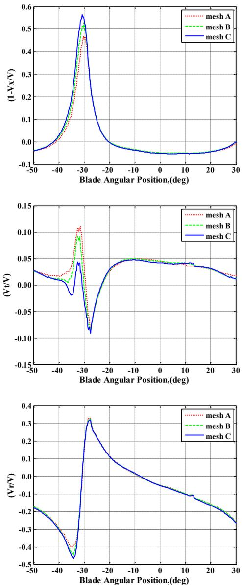
Figure 7: Velocity profiles computed in a plane  $x/D=0.1$  downstream of the propeller mid plane at  $r/R=1$ .
