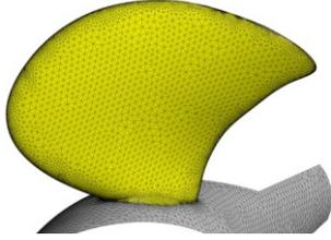
Figure 3: Hybrid blade surface mesh
