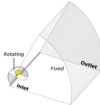
Figure 5: Computational Domain for Cavitation Tunnel Test
