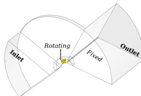
Figure 2: Computational domain for the Towing tank tests
