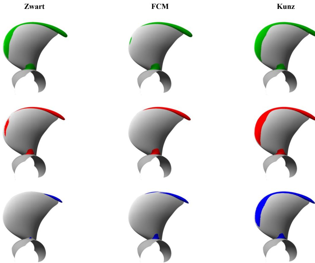
Figure 9: Cavitation patterns predicted for  $J=1.016$ ,  $\sigma_n=2.024$  using different mass transfer models. For each model the cavitation pattern is depicted using three different iso-surfaces of the vapour volume fraction  $\alpha$ ;  $\alpha=0.20$  (green),  $\alpha=0.50$  (red),  $\alpha=0.80$  (blue).
