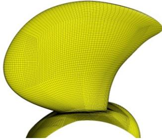
Figure 6: Hexa-structured blade surface mesh
