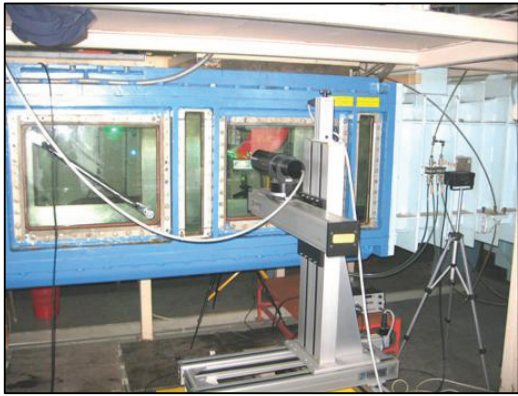
Figure 3 View on test section and LDA equipment
