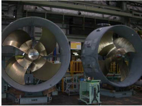
Figure 14 New Designed Ducted Propeller at Full Scale
