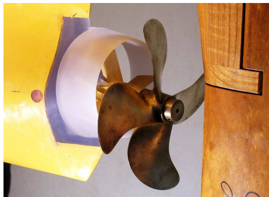
Figure 10 Bulk carrier ship model with installed PSD model, view diagonal from the back/port side, HSVA
