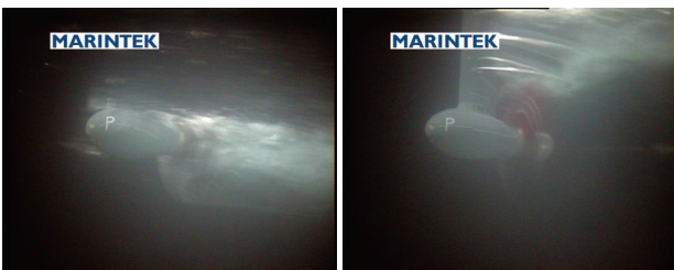
Figure 22 Underwater picture, left: wave trough, right: wave crest, propeller immersion ratio h_0/R=1.2 , advance coefficient J=0.8
