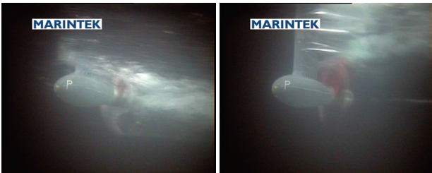
Figure 21 Underwater picture, left: wave trough, right: wave crest, propeller immersion ratio h_0/R=1.6 , advance coefficient J=0.8
