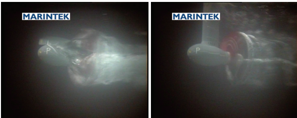
Figure 20 Underwater picture, left: wave trough, right: wave crest, propeller immersion ratio h_0/R=1.2 , advance coefficient J=0.4
