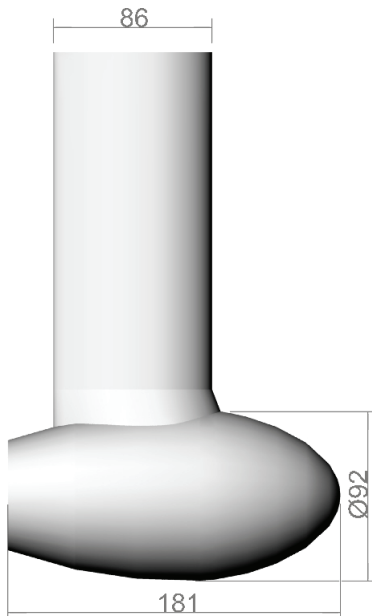
Figure 2 Rendered drawing of thruster body (side view)
