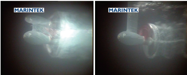
Figure 19 Underwater picture, left: wave trough, right: wave crest, propeller immersion ratio h_0/R=1.6 , advance coefficient J=0.4
