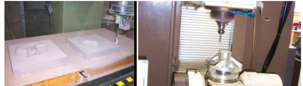
Figure 6 Ureal moulds for blank casting and prototype machining
