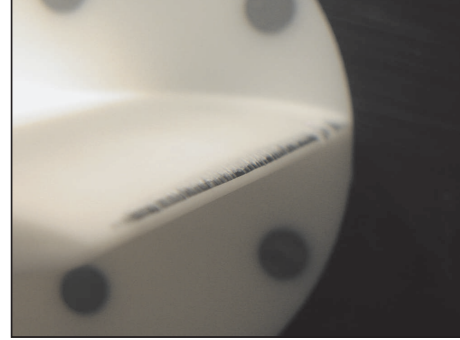
Figure 10. Cavitation inception at the leading edge for a fixed angle of incidence, \alpha = 8^\circ , \sigma = 3
