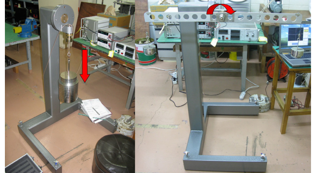
Figure 2 Calibration stand for propeller dynamometer
