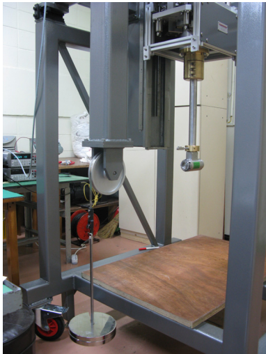
Figure 6 Calibration of balance with offset position
