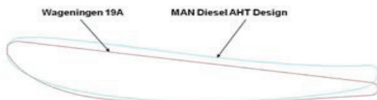
Figure 1: Comparison between 19A and AHT nozzle profile
