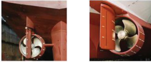
Figure 3: Typical strut and head-box arrangement
