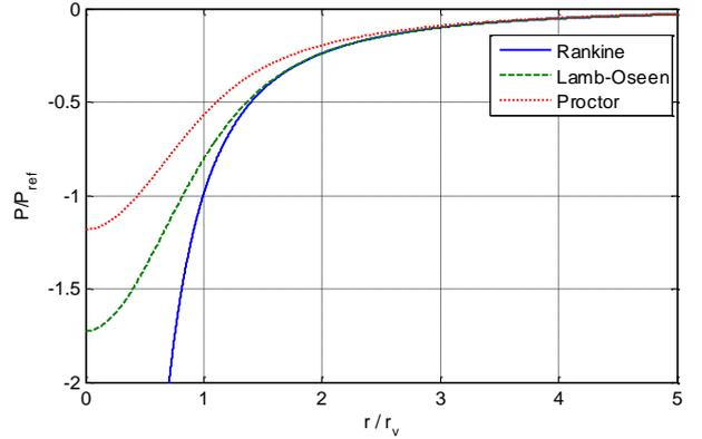
Figure 2. Non-dimensional pressure distribution for various vortex models.
