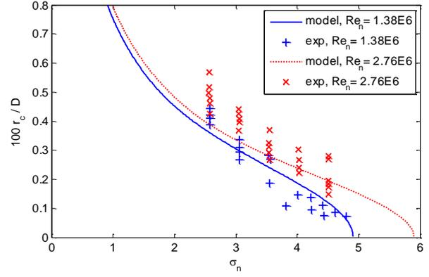
**Figure 4.** Measured and fitted variation of cavity size for a propeller at advance ratio  $J= 0.4$ . Experiments by Kuiper (1981).
