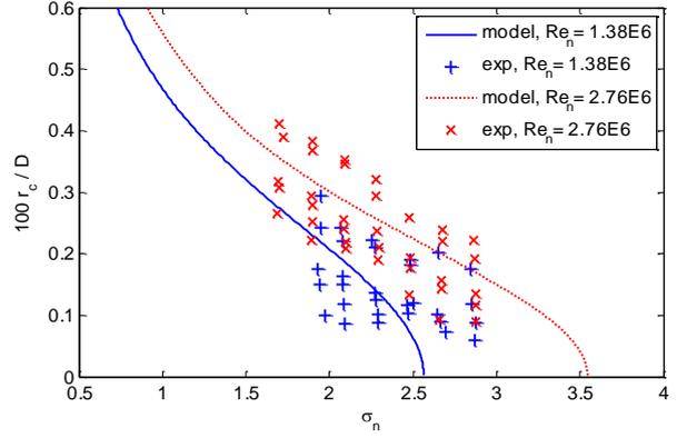
**Figure 5.** Measured and fitted variation of cavity size for a propeller at advance ratio  $J= 0.5$ . Experiments by Kuiper (1981).
