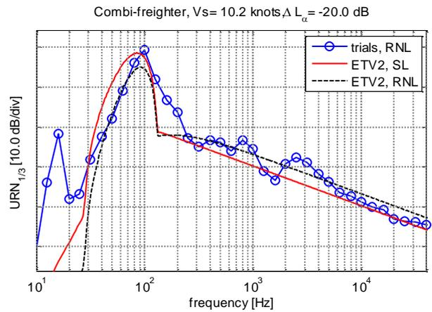
**Figure 17. Measured and predicted radiated noise spectrum in one-third octave band levels for the combi-freighter using adapted value for  $\Delta L_\alpha$ .**
