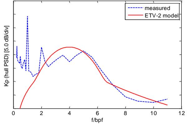
Figure 14. Example of the measured and predicted non-dimensional hull pressure spectrum for a ship propeller of the database tested at full scale.
