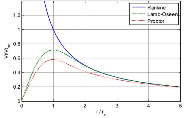
Figure 1. Non-dimensional azimuthal velocity distribution for various vortex models.
