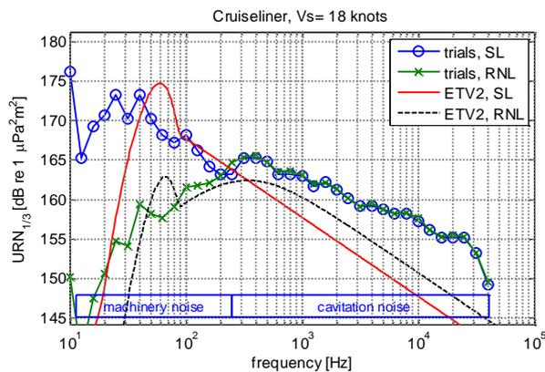
**Figure 18. Measured and predicted radiated noise spectrum in one-third octave band levels for the cruise vessel using default values for the prediction model.**
