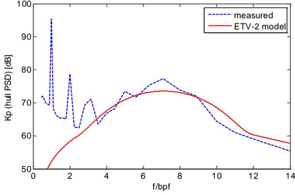
Figure 12. Example of the measured and predicted non-dimensional hull pressure spectrum for a two-bladed research propeller.
