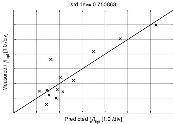
**Figure 8. Comparison between measured and predicted center frequencies for propellers dominated by tip vortex cavitation.**
