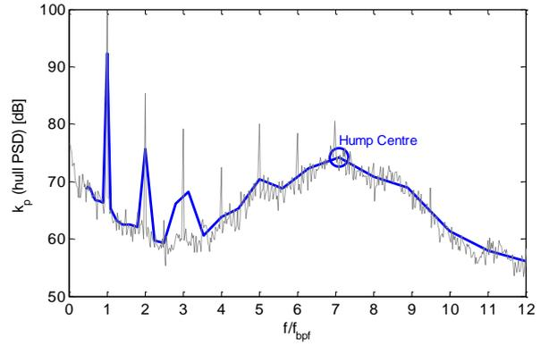
**Figure 6. Example of a non-dimensional hull pressure power density spectrum of a two bladed research propeller. The solid line is the 1/6 octave band smoothed spectrum.**
