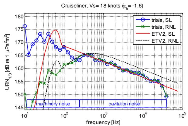
**Figure 19. Measured and predicted radiated noise spectrum in one-third octave band levels for the cruise vessel using adapted values for the high frequency slope parameter  $\alpha_h$ .**
