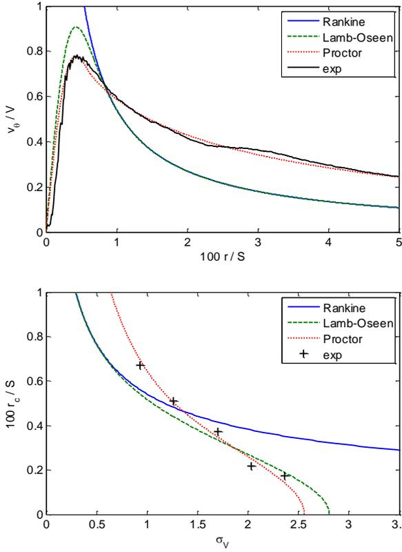
**Figure 3.** Measured and fitted azimuthal velocity distribution (top) and cavity size variation (bottom) for a wing of elliptical planform at 7 deg angle of attack. Experiments by Pennings *et al.* (2015b).
