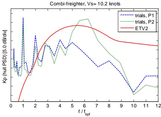
**Figure 15. Measured and predicted non-dimensional hull pressure spectrum for the combi-freighter. P1 corresponds to the center transducer and P2 is located closer to the cavity collapse.**
