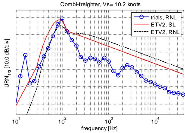
**Figure 16. Measured and predicted radiated noise spectrum in one-third octave band levels for the combi-freighter using default values for the prediction model.**
