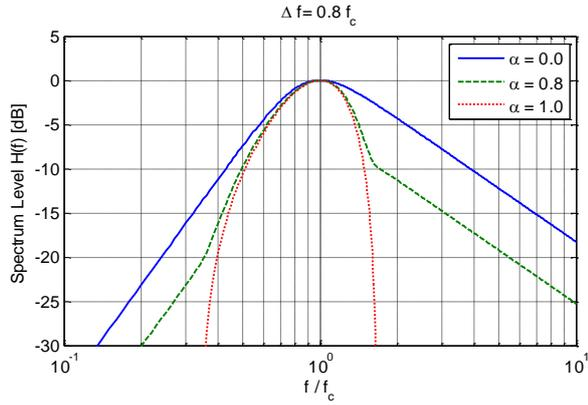
**Figure 10.** Examples of the shape of the spectrum for different values of  $\alpha$ .
