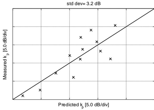
**Figure 7. Comparison between measured and predicted center level of the hump for propellers dominated by tip vortex cavitation.**
