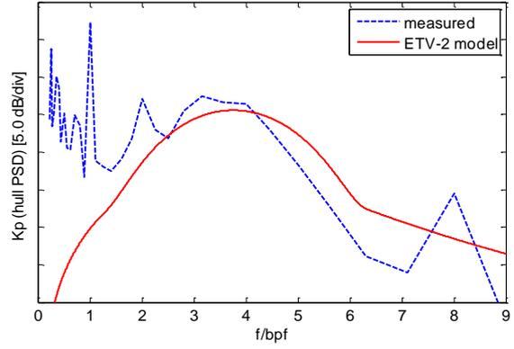
Figure 13. Example of the measured and predicted non-dimensional hull pressure spectrum for a ship propeller of the database tested at model scale.
