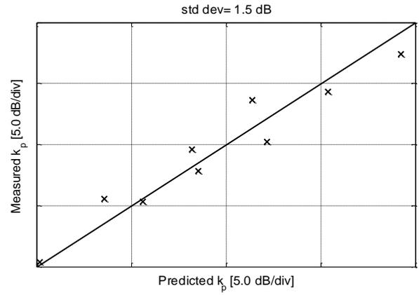
**Figure 9. Comparison between measured and predicted center level of the hump for a two-bladed research propeller tested at various advance ratios and cavitation numbers.**
