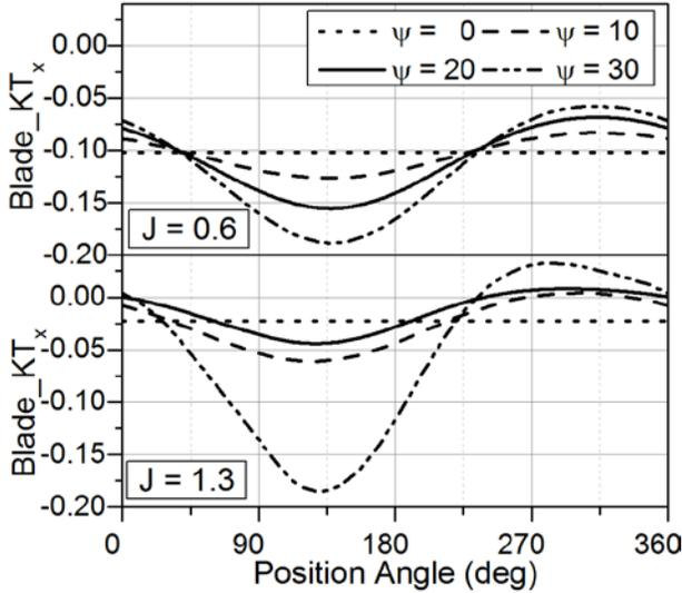
**Figure 8:** Longitudinal blade forces, expressed as a  $K_T$  coefficient as a function of blade position, for discretized geometry, at different shaft angles. Top panel  $J = 0.6$ ; lower panel  $J = 1.3$ .
