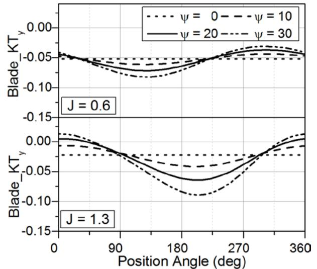
**Figure 11:** Lateral (y) blade forces, expressed as a  $K_T$  coefficient as a function of blade position, for PUF-14 modelled propeller, at different shaft angles. Top panel  $J = 0.6$ ; lower panel  $J = 1.3$ .
