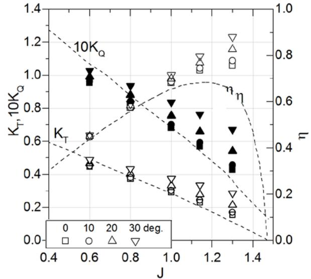
**Figure 7:** Open water curves for propeller P4661 at different shaft angles with respect to the carriage advance direction. Blades simulated using PUF-14 model. Dotted lines correspond to experimental values at 0 degrees. Solid symbols correspond to  $K_Q$ , thick line symbols to  $K_T$  and thin line symbols to  $\eta$ . The shaft angle is described in the plot legend.
