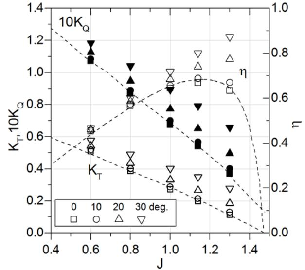
**Figure 6:** Open water curves for propeller P4661 at different shaft angles with respect to the carriage advance direction. Blades simulated using discretized geometry. Dotted lines correspond to experimental values at 0 degree. Solid symbols correspond to  $K_Q$ , thick line symbols to  $K_T$  and thin line symbols to  $\eta$ . The shaft angle is described in the plot legend.
