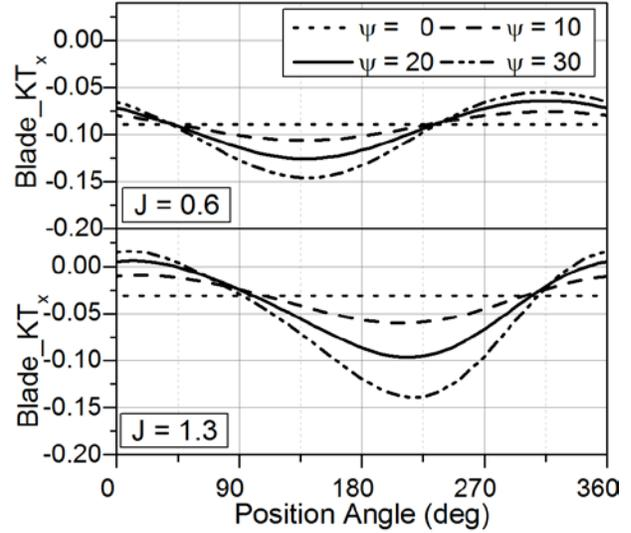
**Figure 10:** Longitudinal blade forces expressed as a  $K_T$  coefficient as a function of blade position, for PUF-14 modelled propeller, at different shaft angles. Top panel  $J = 0.6$ ; lower panel  $J = 1.3$ .
