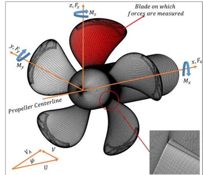
**Figure 2:** Domain and coordinates convention for propeller P4661 open water simulations.
