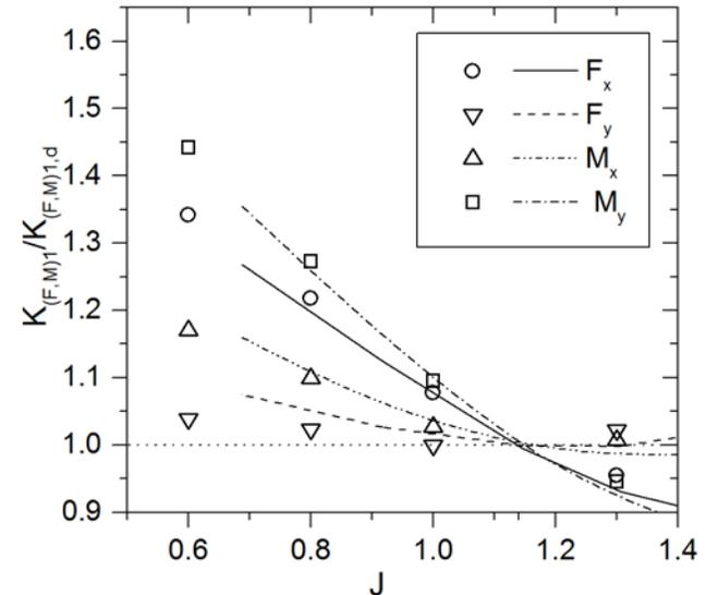
**Figure 14:** Amplitude of the first harmonic as a fraction of the value near design  $J$  for longitudinal and lateral forces and moments for direct method at shaft angle 20 degrees. Lines correspond to experimental values from Boswell *et al.* (1981) and symbols to direct method simulations.
