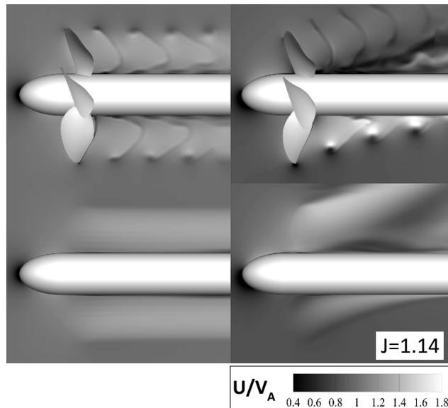
**Figure 3:** Longitudinal fluid velocity at advance coefficient  $J = 1.14$  (design value). Top: discretized blades; bottom PUF-14 modelled propeller. Shaft angle is zero for left column and 30 degrees for right column plots. Velocity is non-dimensionalized with carriage advance velocity.
