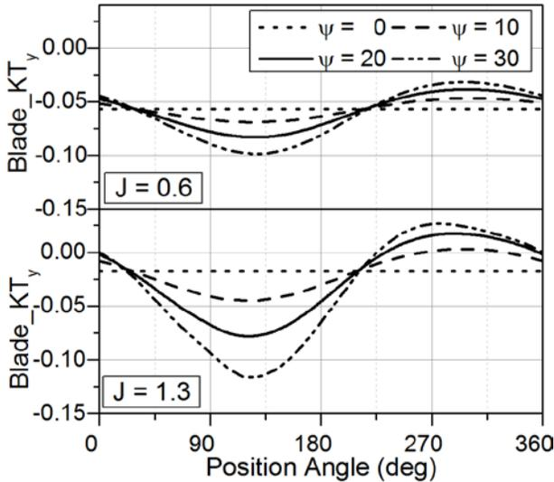
**Figure 9:** Lateral (y) blade forces, expressed as a  $K_T$  coefficient as a function of blade position, for discretized geometry, at different shaft angles. Top panel  $J = 0.6$ ; lower panel  $J = 1.3$ .
