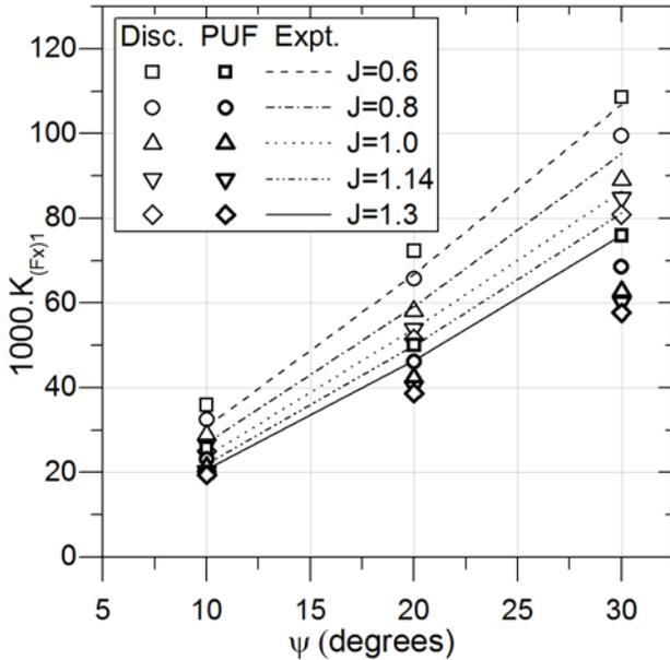
**Figure 12:** Amplitude of the first harmonic for propeller P4661 at different shaft angles with respect to the carriage advance direction. Blades simulated using PUF-14 model. Lines correspond to experimental values, and symbols to discretized or modelled blades as shown in plot legend. Experimental values are interpolated (and for  $J=0.6$ , extrapolated) to reconcile the different definitions of the advance velocity between experiments and simulations.
