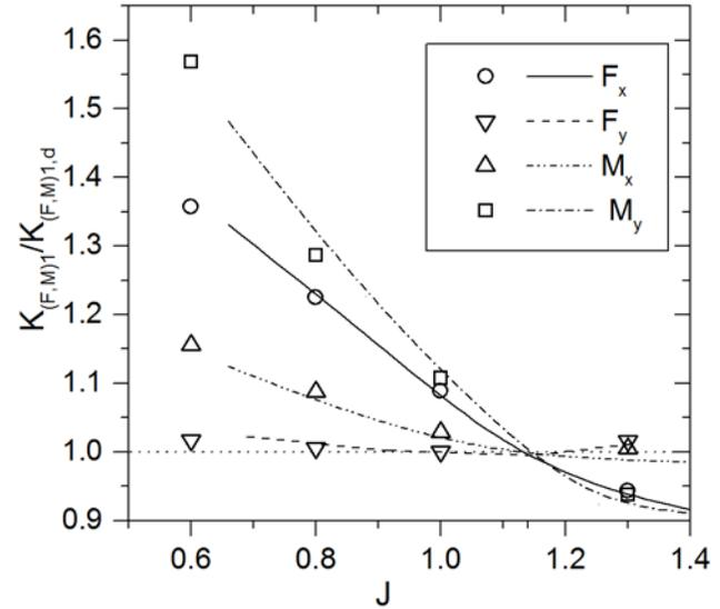
**Figure 13:** Amplitude of the first harmonic as a fraction of the value near design  $J$  for longitudinal and lateral forces and moments for direct method at shaft angle 10 degrees. Lines correspond to experimental values from Boswell *et al.* (1981) and symbols to direct method simulations.
