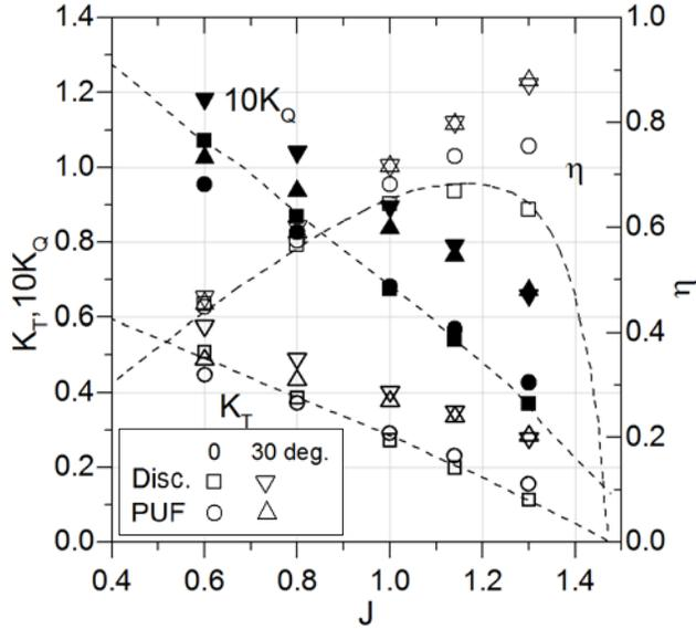
**Figure 5:** Open water curves for propeller P4661 at 0 and 30 degree shaft angles with respect to the carriage advance direction. Discretized geometry and coupled model results are shown. Dotted lines correspond to experimental values at 0 degrees. Solid symbols correspond to  $K_Q$ , thick line symbols to  $K_T$  and thin line symbols to efficiency. The model used and shaft angle are described in the plot legend.
