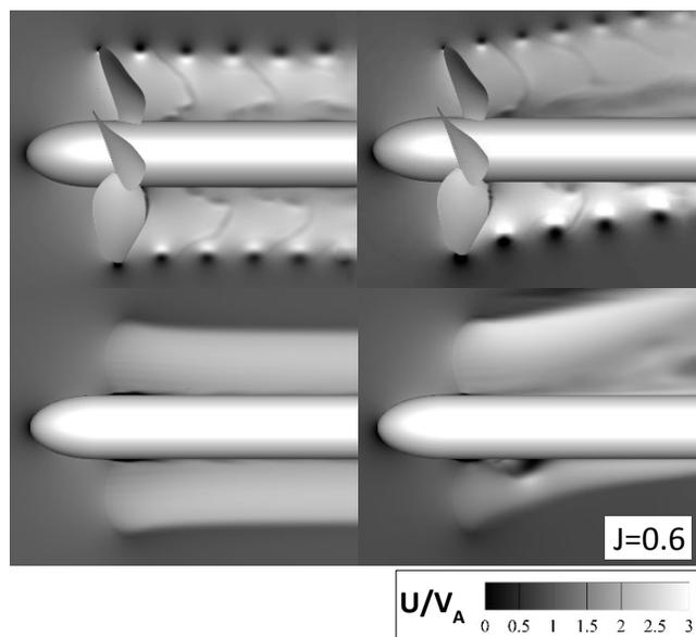
**Figure 4:** Longitudinal fluid velocity at advance coefficient  $J = 0.6$ . Top: discretized blades; bottom PUF-14 modelled propeller. Shaft angle is zero for left column and 30 degrees for right column plots. Velocity is non-dimensionalized with carriage advance velocity.
