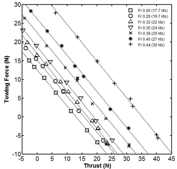
**Figure 9:** Towing force plotted against the propeller thrust for the 130m propeller driven catamaran with the displacement of 3,640 tonnes.
