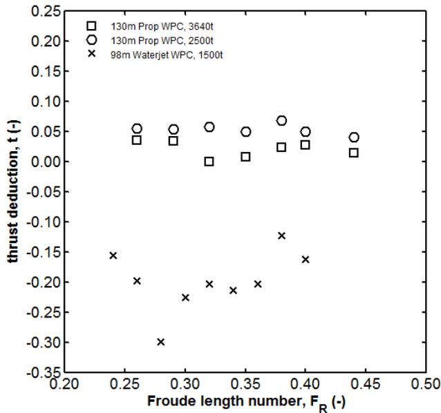
Figure 13: The thrust deduction fractions versus Froude length number.
