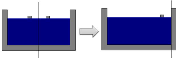
**Figure 1:** Schematic catamaran and equivalent demihull arrangement in towing tank.
