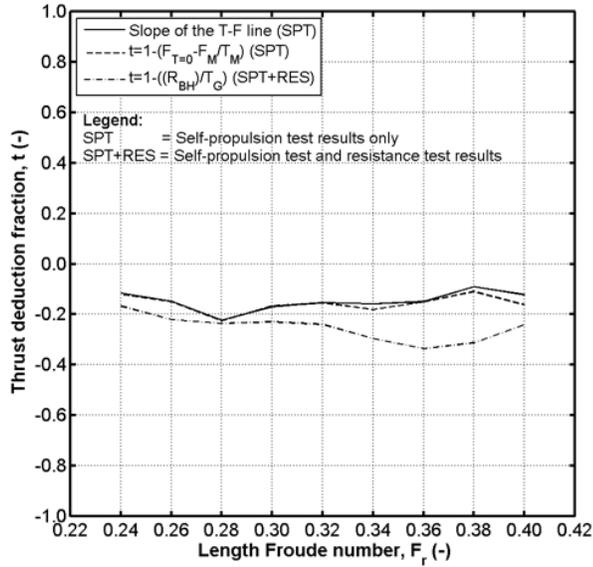
**Figure 1** Comparison of thrust deduction results calculated using bare-hull resistance test results together with waterjet self-propulsion test results and thrust deduction calculated using only waterjet self-propulsion test results.
