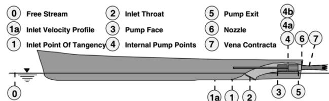
**Figure 5:** Momentum flux method reference stations as defined Final Report and Recommendations to the 23<sup>rd</sup> ITTC.
