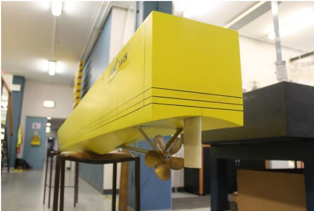
**Figure 3:** The propeller arrangement (with a support bracket and a rudder) of the 130m propeller driven catamaran model
