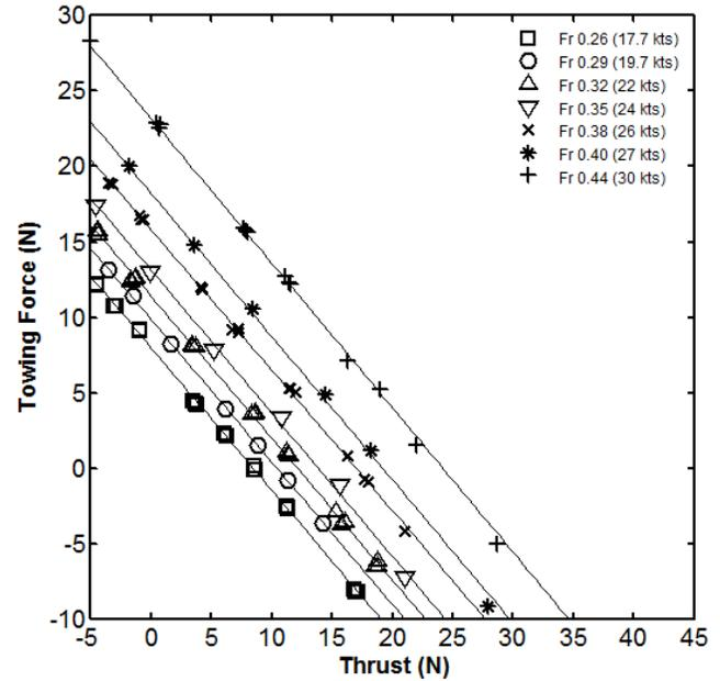
**Figure 8:** Towing force plotted against the propeller thrust for the 130m propeller driven catamaran with the displacement of 2,500 tonnes.
