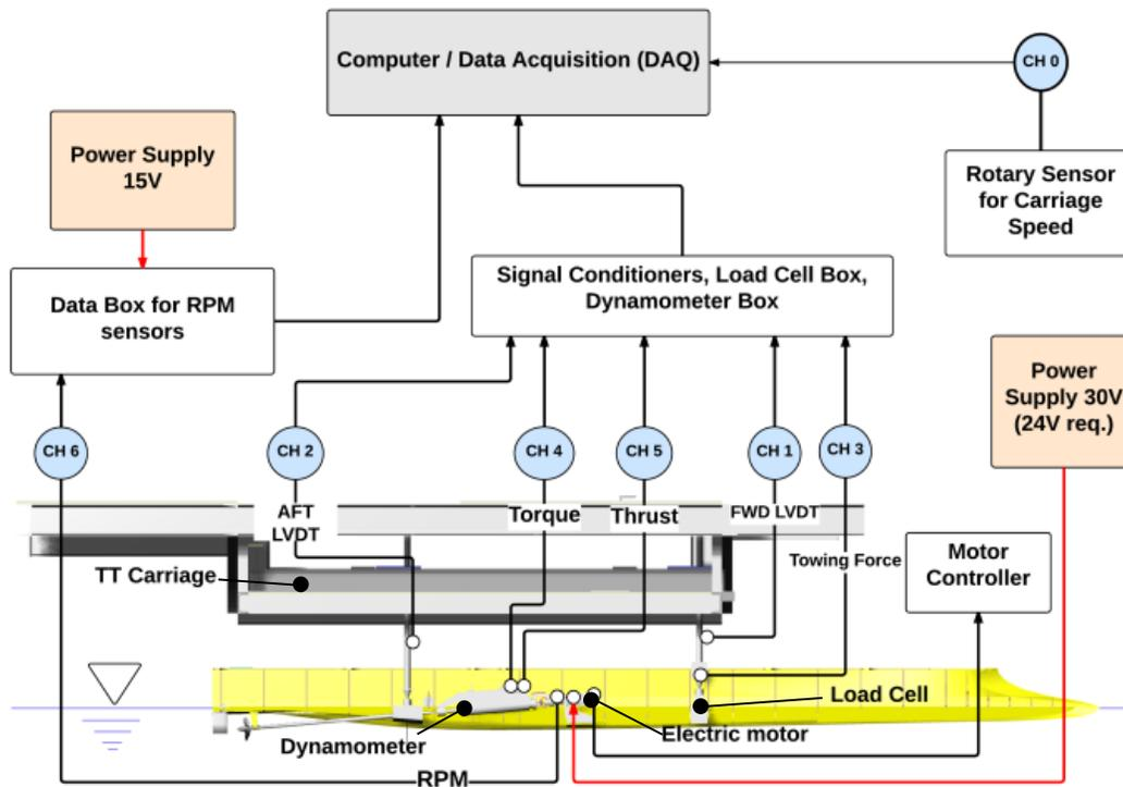
Figure 6: Data acquisition setup for the propeller driven self-propulsion test.
