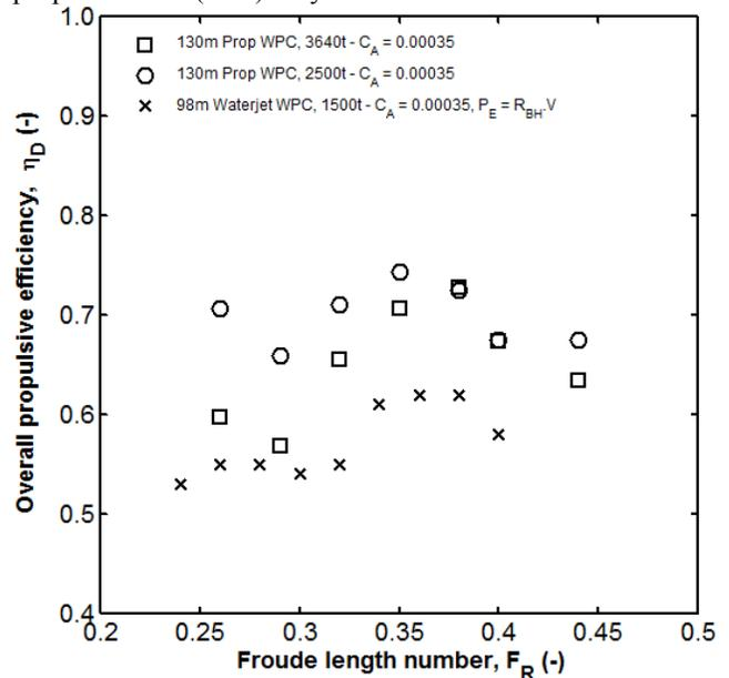
**Figure 12:** Overall propulsive efficiency versus Froude length number. This plot shows the results for the propeller driven and the waterjet driven catamaran.
