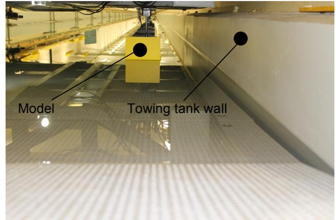
**Figure 2:** The single demihull model of the catamaran in the towing tank in close proximity with the towing tank wall.
