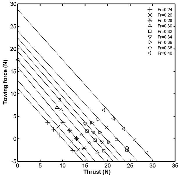
**Figure 10:** Towing force plotted against the propeller thrust for the 98m waterjet driven catamaran with the displacement of 1,500 tonnes.
