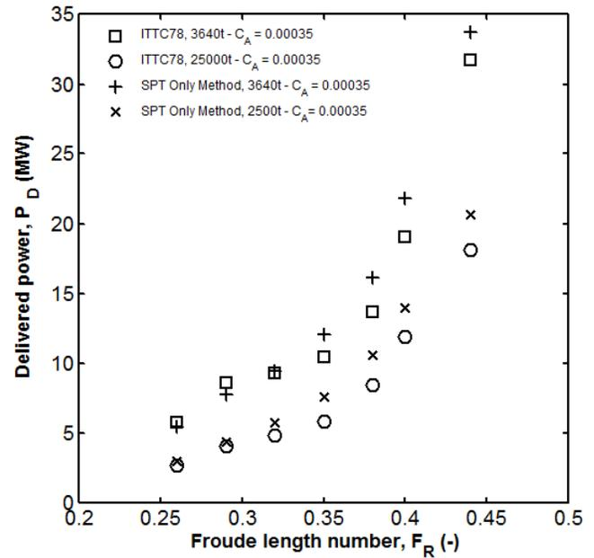
**Figure 11:** The delivered power versus Froude length number for the displacement of 3640 tonnes. The results were extrapolated using the ITTC 1978 method and the self-propulsion test (SPT) only method.
