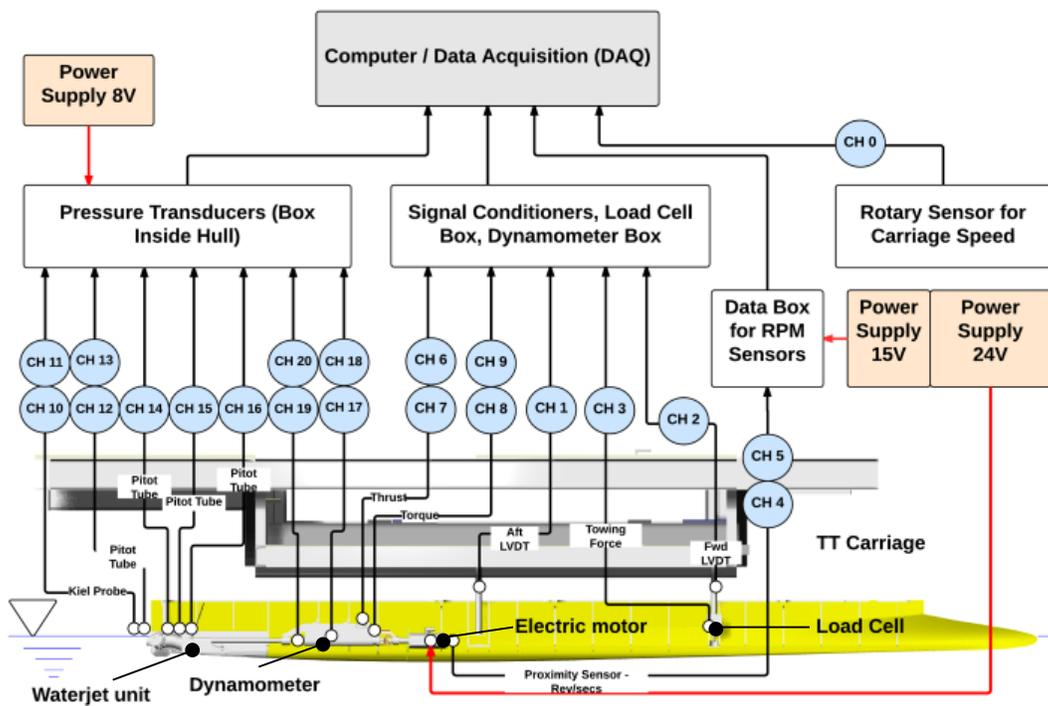
Figure 7: Data acquisition setup for the waterjet driven self-propulsion test.
