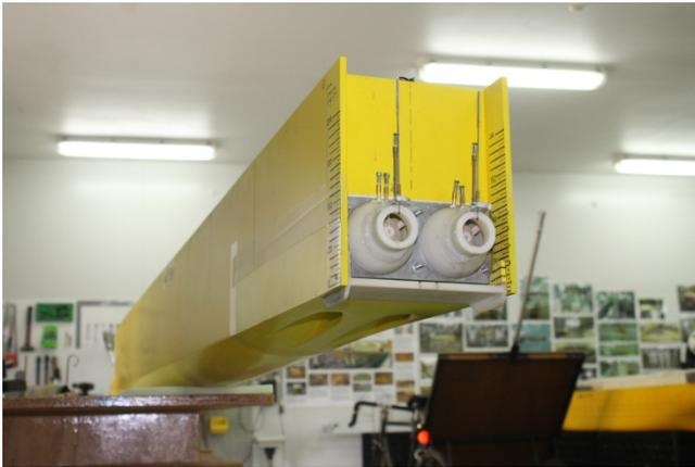
**Figure 4:** The 3D printed waterjet propulsion unit attachment. Note the nozzles and the tunnels of the waterjet unit of the 98m waterjet driven catamaran model.
