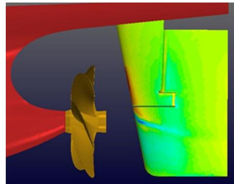
**Figure 21.** Erosion damage predicted by Function 1.
