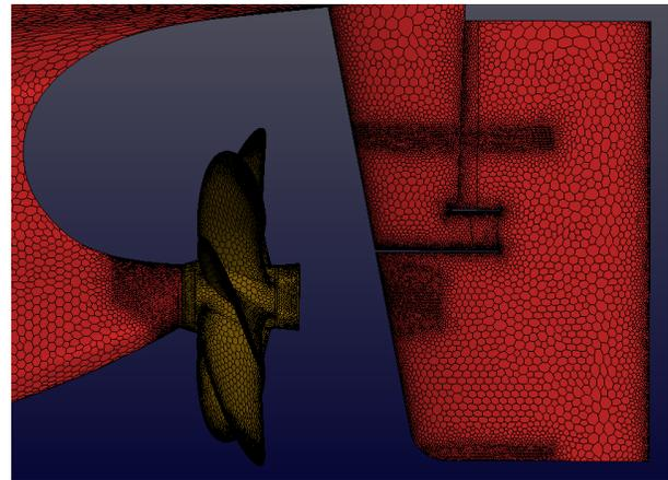
**Figure 15.** Computational mesh on the propeller and rudder.
