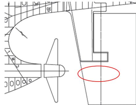
**Figure 20.** Schematic area of observed erosion damage.
