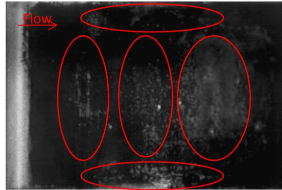
**Figure 8.** Paint removal after the model tests.
