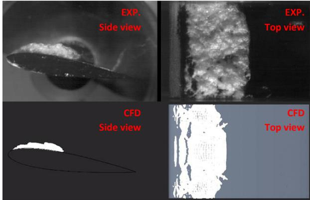
**Figure 3.** Cavitation predicted by CFD vs Experimental observation. Solution time 0.084415 s.
