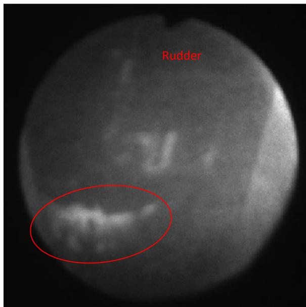
**Figure 19.** Paint damage on the port side of the rudder observed from the borescope position 2.
