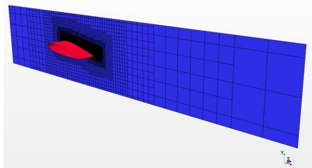
**Figure 1.** Computational domain identical to cavitation tunnel working section.
