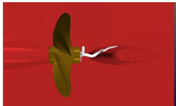
**Figure 17.** Hub vortex predicted by DES. Bottom view.
