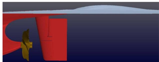
**Figure 14.** Ship scale stern wave.
