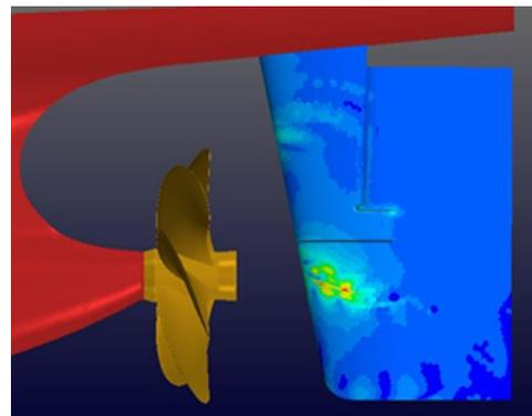
**Figure 22.** Erosion damage predicted by Function 5.
