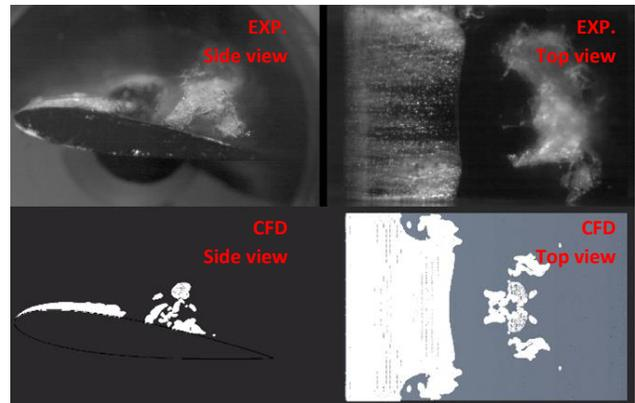
**Figure 7.** Cavitation predicted by CFD vs Experimental observation. Solution time 0.087245 s.
