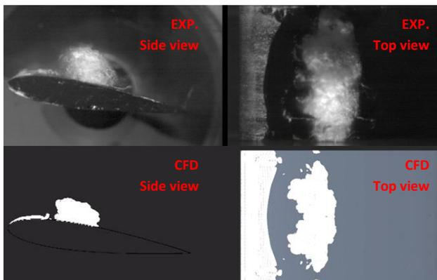
**Figure 5.** Cavitation predicted by CFD vs Experimental observation. Solution time 0.085595 s.
