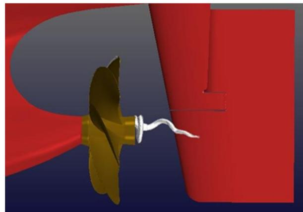
**Figure 16.** Hub vortex predicted by DES. Port side view.
