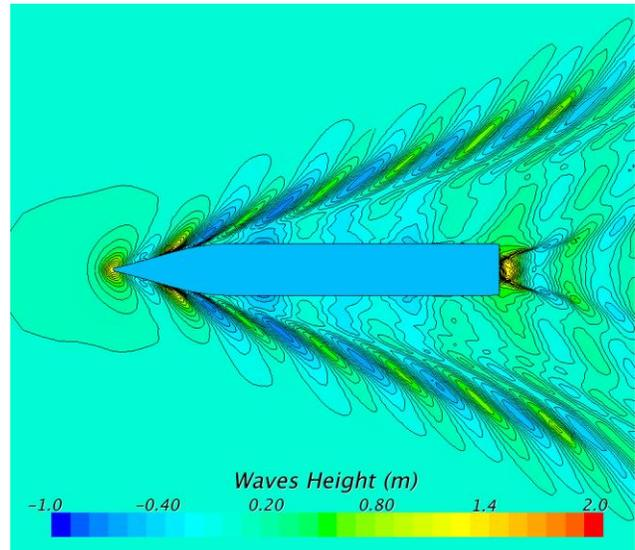
**Figure 13.** Ship scale free surface pattern.
