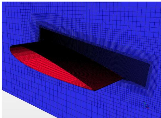
**Figure 2.** Mesh refinement above the foil.
