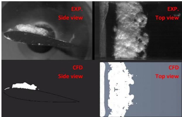
**Figure 4.** Cavitation predicted by CFD vs Experimental observation. Solution time 0.084825 s.
