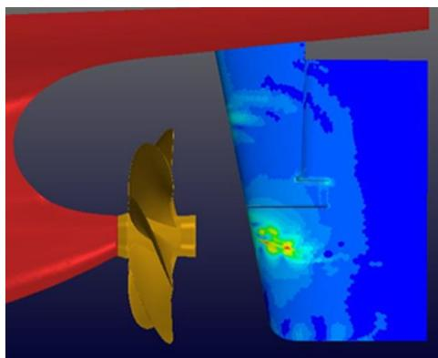
**Figure 23.** Erosion damage predicted by Function 8.
