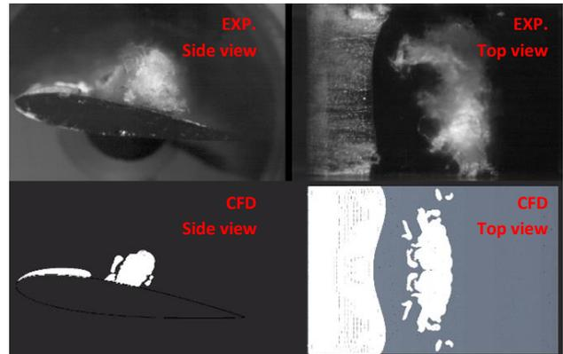
**Figure 6.** Cavitation predicted by CFD vs Experimental observation. Solution time 0.086245 s.
