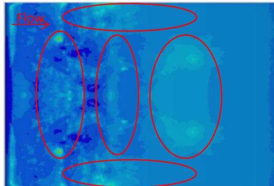
**Figure 10.** Erosion zones predicted by Function 5.
