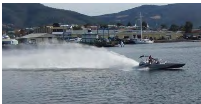
Figure 4 – Trials with flat blade paddle wheel, 32 knots.
