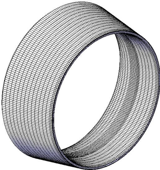
Figure 3: Panel mesh of the duct
