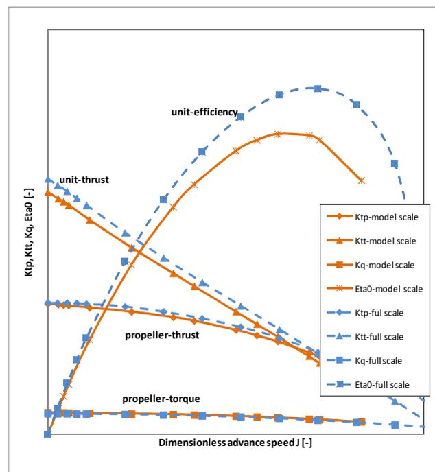
Figure 3: comparison of model scale and full scale CFD results for thruster open water performance
