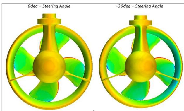
Figure 12: pressure distribution on thruster unit for 0 degree steering (left) and -30 degree steering
