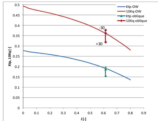
Figure 9: propeller thrust ( $K_{tp}$ ) and torque ( $10K_q$ ) in open water conditions and with oblique inflow
