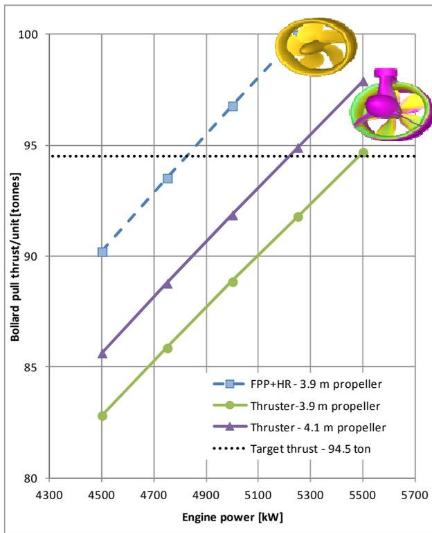
**Figure 6: bollard pull performance prediction for 2 example case studies to analyze effect of thruster house geometry and propeller diameter variation**
