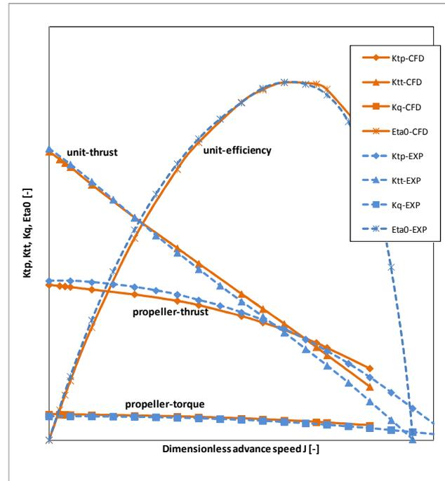
Figure 2: comparison model scale experimental data with model scale CFD results for thruster open water performance
