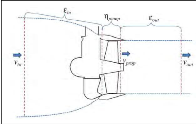
Figure 4: sketch of thruster-unit with merit-coefficient parameters
