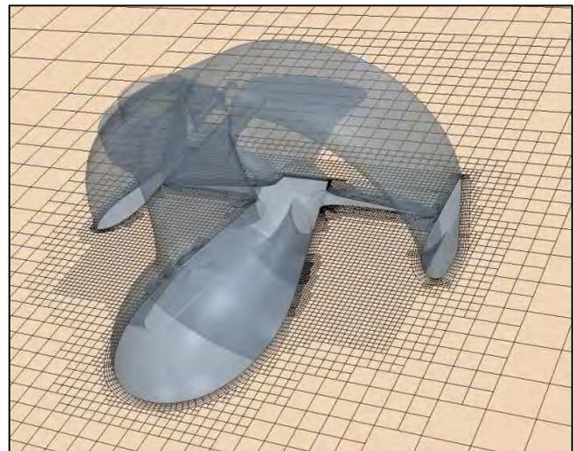
Figure 1: thruster mesh visualization in horizontal plane
