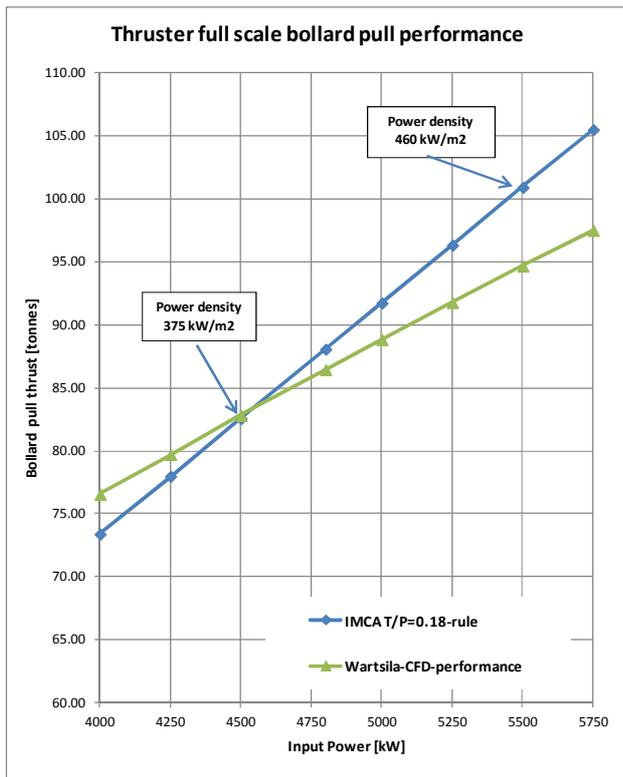
Figure 5: thruster bollard pull comparison based on equations (5) and (6)
