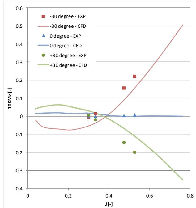
Figure 13: comparison model scale experimental data with model scale CFD results for thruster hydrodynamic steering torque
