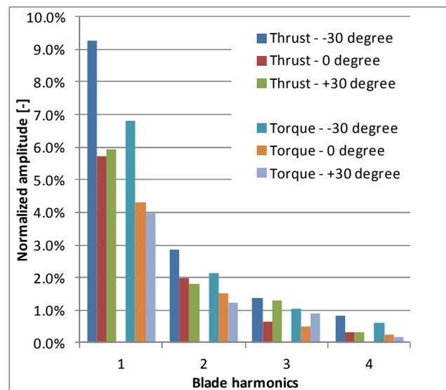
Figure 10: normalized amplitudes of propeller thrust and torque for free sailing with straight and oblique inflow
