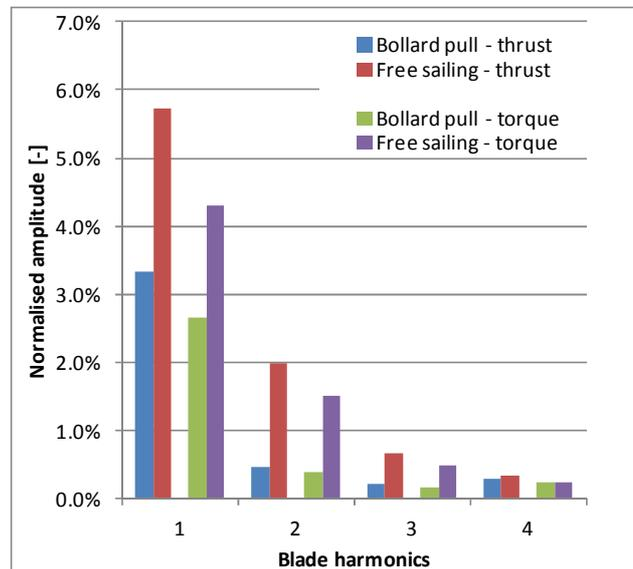
**Figure 7: normalized amplitudes of propeller thrust and torque for bollard pull and free sailing condition**
