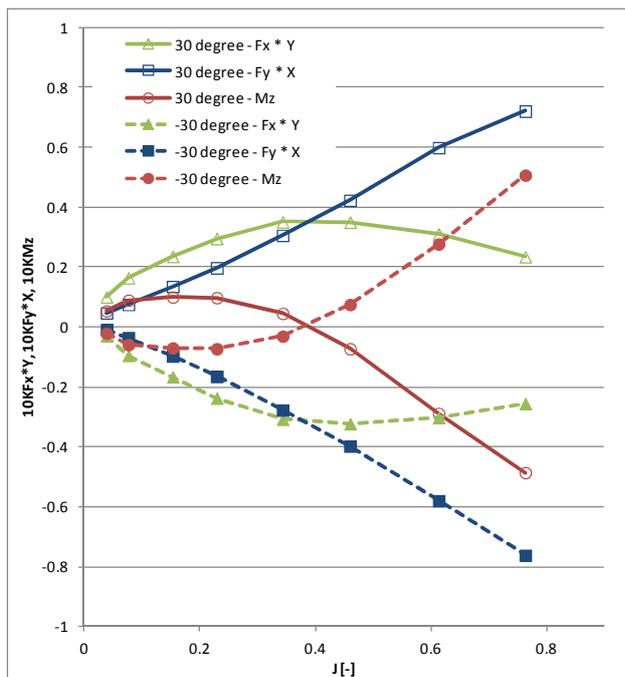
Figure 14: analysis of steering torque components based on equation (7): total steering torque in red, thrust eccentricity in green, side-force in blue. The positive steering angle is shown with solid lines and the negative steering angle with dotted lines.
