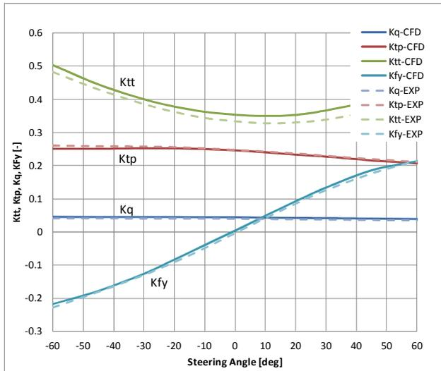
Figure 8: comparison of CFD results (solid lines) and experimental data (dotted lines) for unit thrust ( $K_{tt}$ ), side force ( $K_{fy}$ ), propeller thrust ( $K_{tp}$ ) and torque ( $K_q$ ) for a thruster-unit operated at different oblique inflow angles
