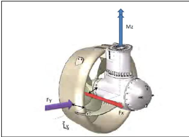
Figure 11: sketch of thruster with contributing forces to hydrodynamic steering torque
