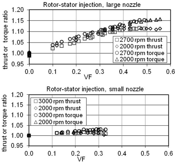
Figure 6: Rotor-stator injection effects on thrust and torque
