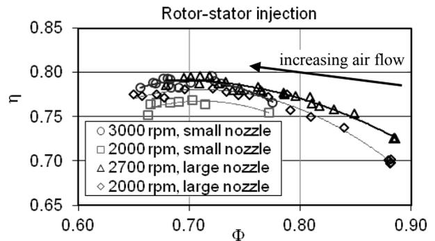
Figure 9: Pump (rotor headrise) efficiency vs flowrate
