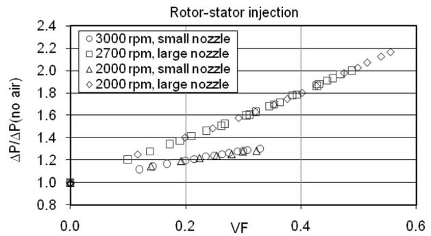
Figure 8: Rotor-stator injection effects on rotor headrise
