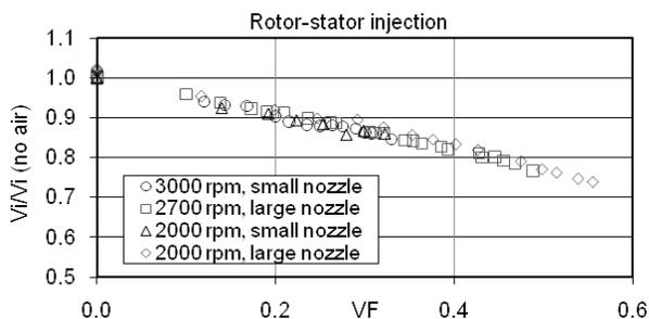
Figure 7: Rotor-stator injection effects on pump flowrate
