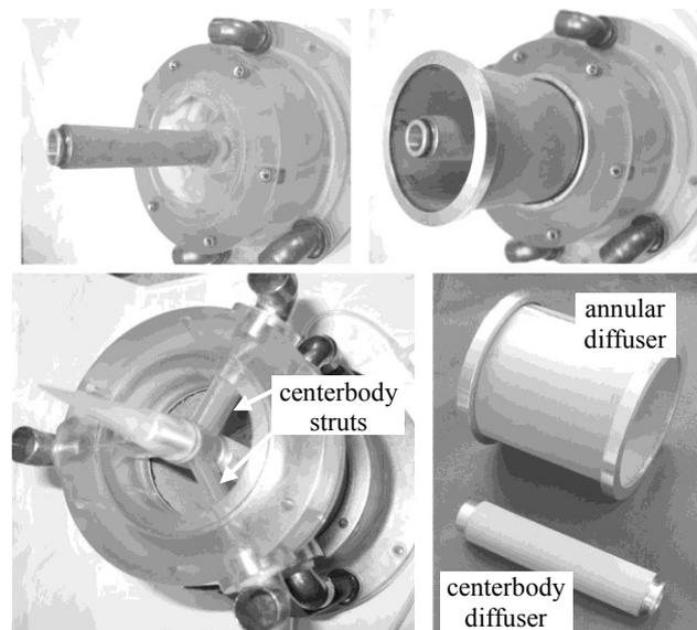
Figure 3: Post stator injector assembly
