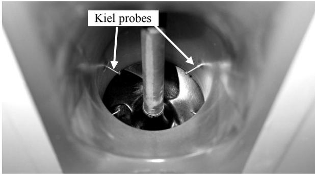
Figure 4: Kiel probes in inlet
