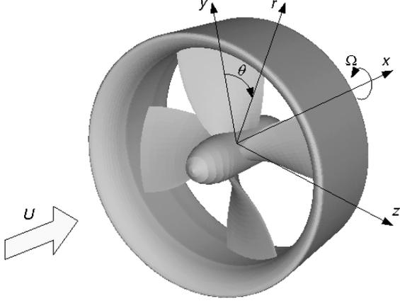
Figure 1: Propeller coordinate system.
