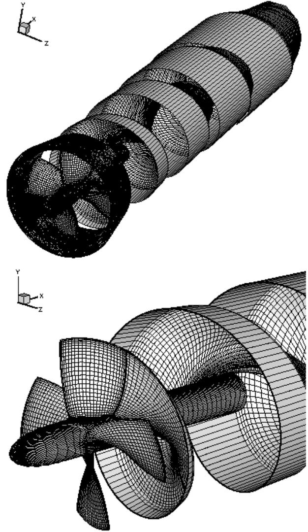
Figure 9: Panel arrangement for propeller Ka4-70 inside duct 19Am at  $J = 0.5$ . Gap model with transpiration velocity. Wake alignment model with duct boundary layer correction. The duct grid is not shown in the bottom figure.
