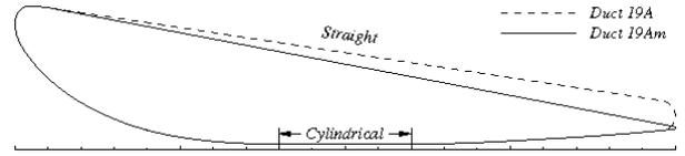
Figure 2: Profiles of duct 19A and 19Am.
