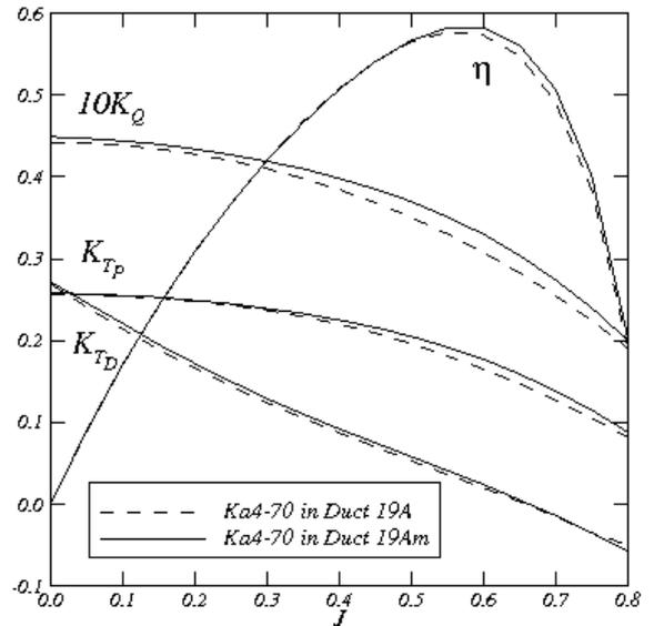
Figure 3: Experimental open-water characteristics of propeller Ka4-70 in duct 19A and duct 19Am.
