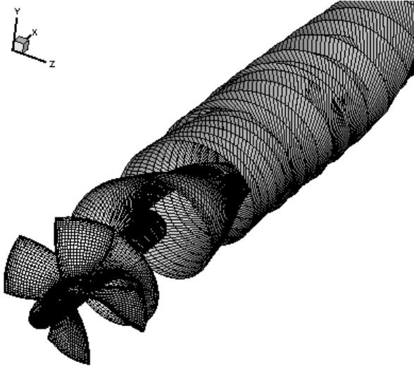
Figure 6: Panel arrangement for propeller Ka4-70 at  $J = 0.5$  for the wake alignment model with empirical contraction. Note that the only one blade wake grid ( $400 \times 25$ ) is shown.
