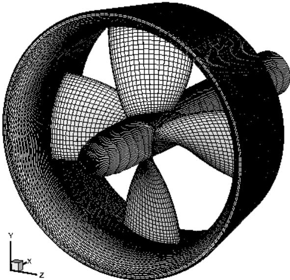
Figure 4: Panel arrangement for propeller Ka4-70 inside duct 19Am. 50×25 panels on each blade; 142×160 panels on the duct; 55×80 panels on the hub.
