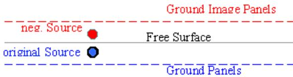
**Figure 1: Current approach for the simulation of shallow water conditions in principle (omitting the hull panel system): every singularity or boundary shows a negative image above the free surface.**
