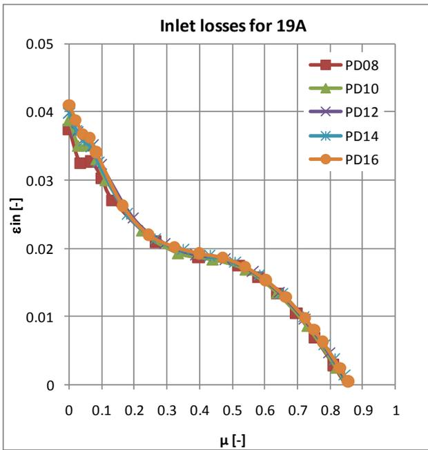
**Figure 5: Inlet loss-coefficient  $\epsilon_{in}$  for different propellers in 19A nozzle**
