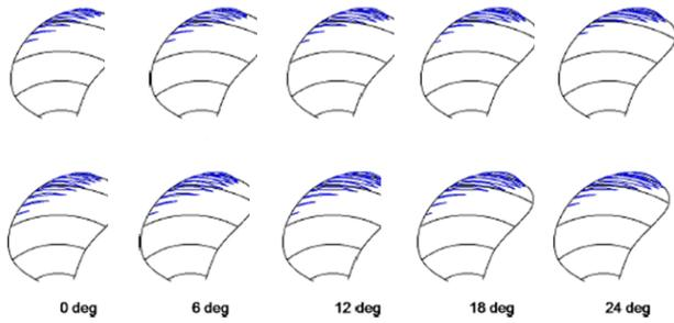
**Figure 12: Comparison of calculated cavity extent based on measured (top) and calculated wakefield on model scale**
