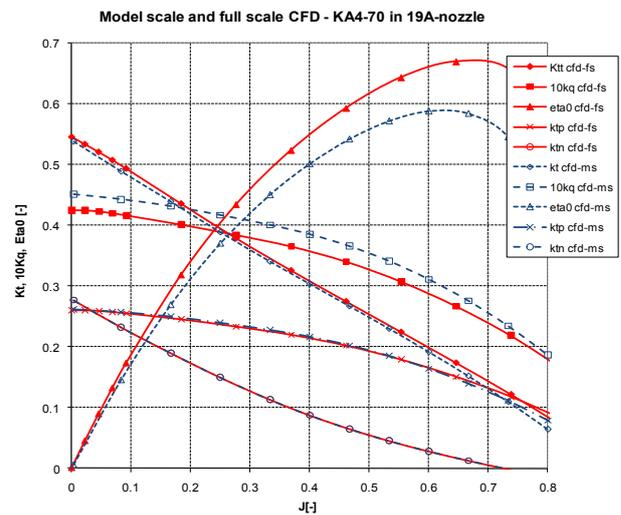
**Figure 3: Comparison of calculated open water performance of Kaplan 4-70 propeller in 19A nozzle on model scale and full scale**
