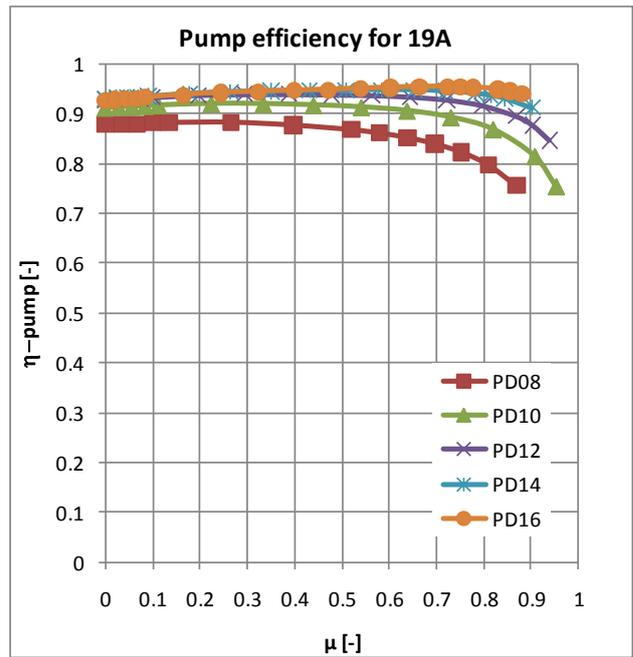
**Figure 7: Pump efficiency for propellers with different P/D-ratios in 19A-nozzle**
