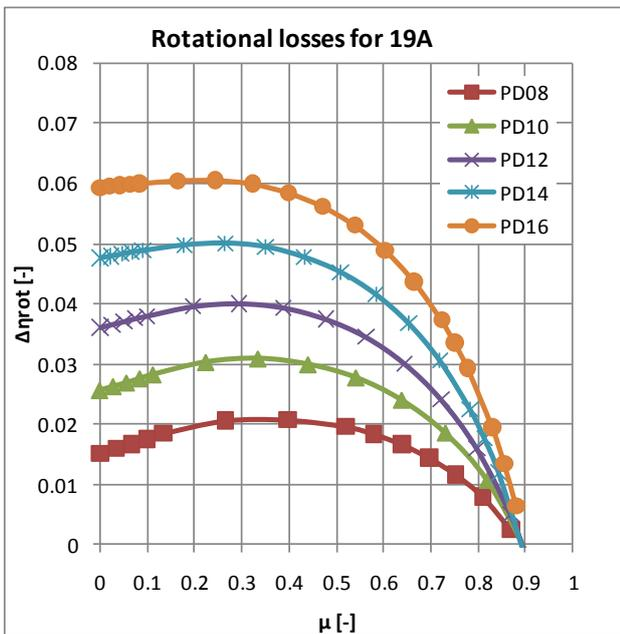
**Figure 6: Rotational loss for different propellers in 19A nozzle**
