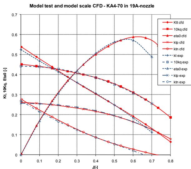
**Figure 2: Comparison of measured and calculated open water performance of Kaplan 4-70 propeller in 19A nozzle**
