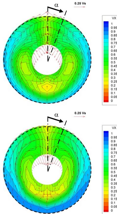
Figure 11: Comparison of measured (top) and calculated wakefield on model scale
