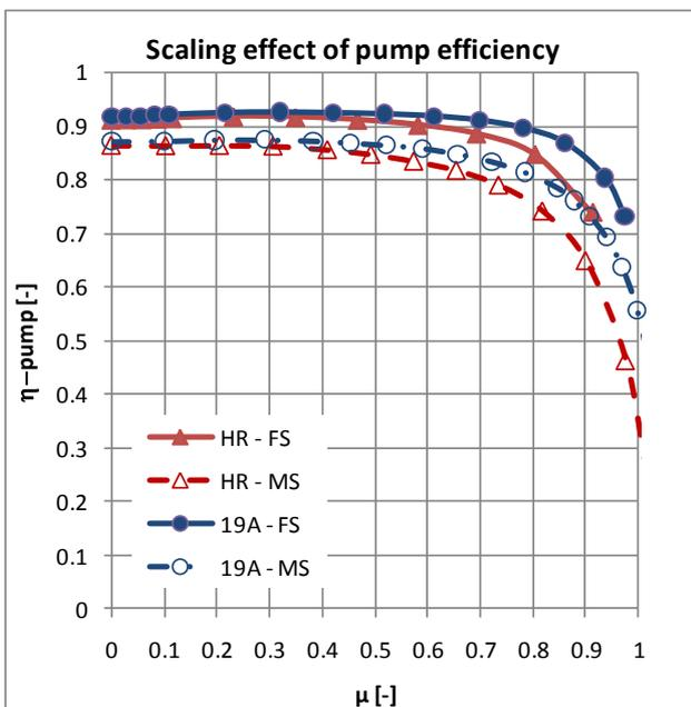
Figure 9: Comparison of pump efficiency for model scale and full scale for 19A and HR nozzle
