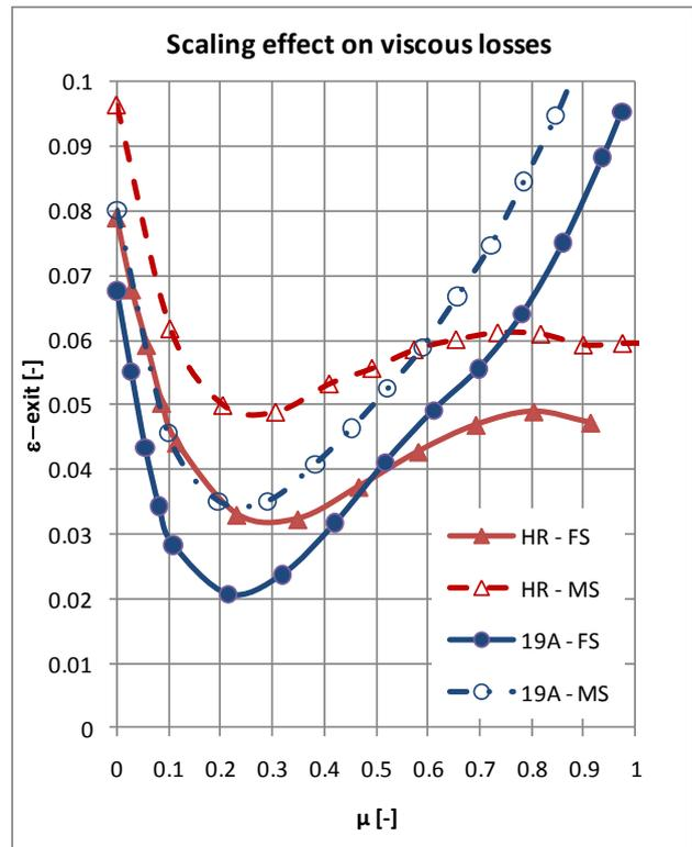
Figure 10: Comparison of loss coefficients for model scale and full scale for 19A and HR nozzle
