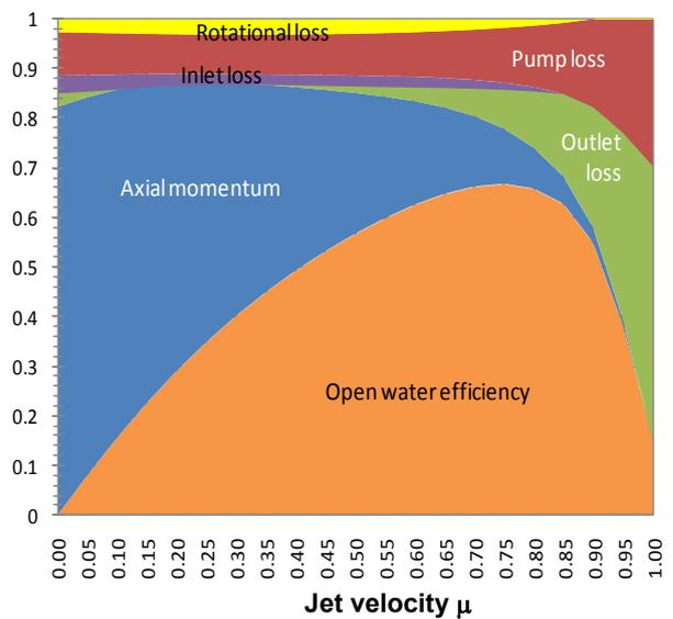
**Figure 8: Overview of all loss coefficients over jet velocity range  $\mu$**
