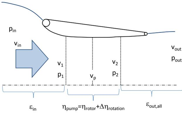
**Figure 4: Sketch of parameters used in ducted-propeller post-processing**
